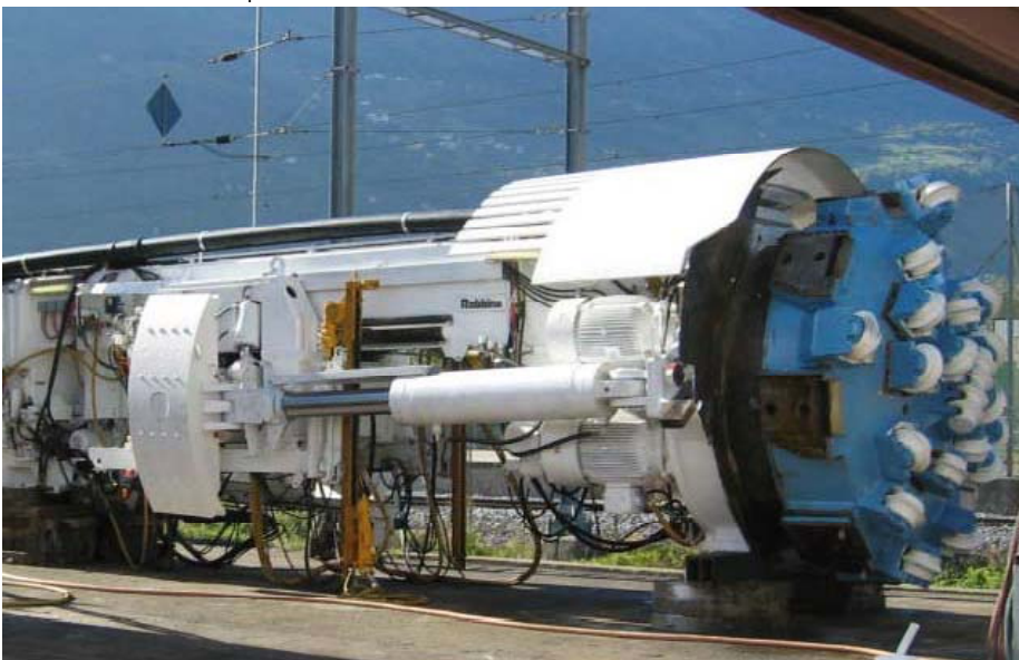
Figure 16. Hard rock TBM diameter 3.8m courtesy by Robbins Company
