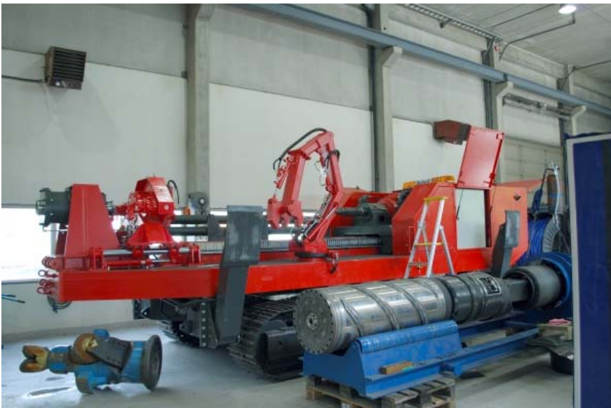
Figure 17. Norhard equipment for drilling 700 mm directional drill hole (Photo: www.norhard.no )
